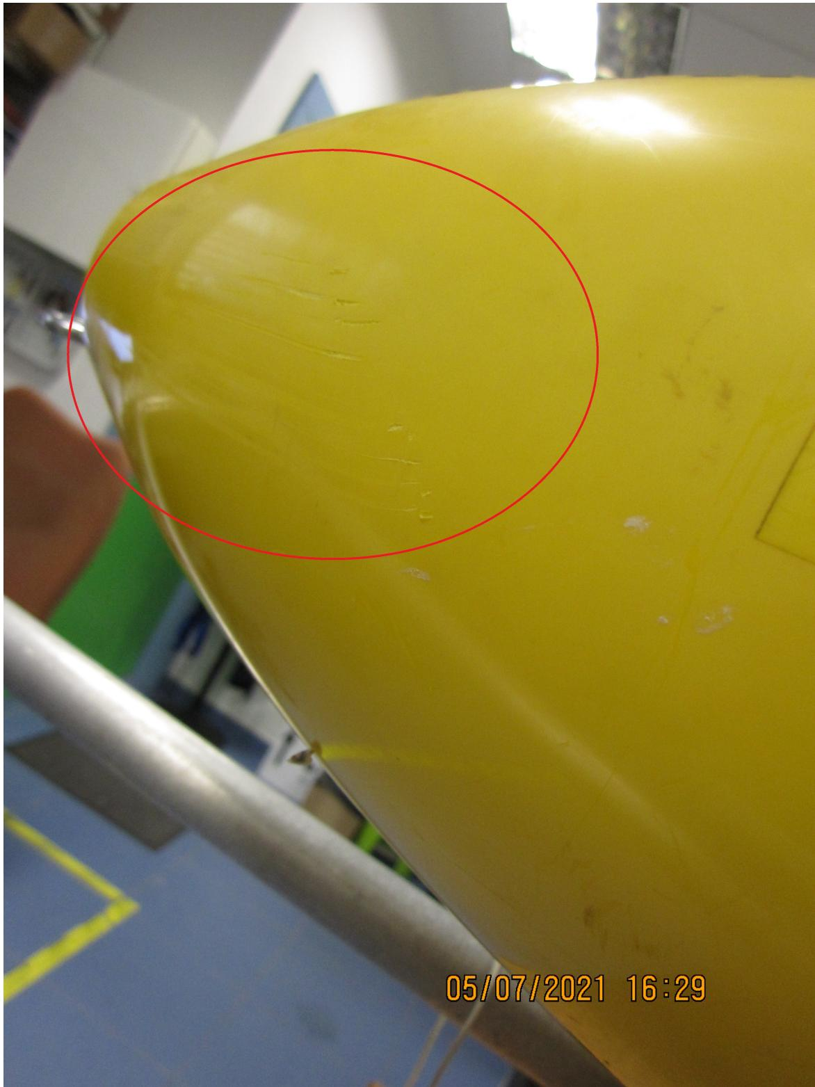
Figure 2.1: Hull Scratches
