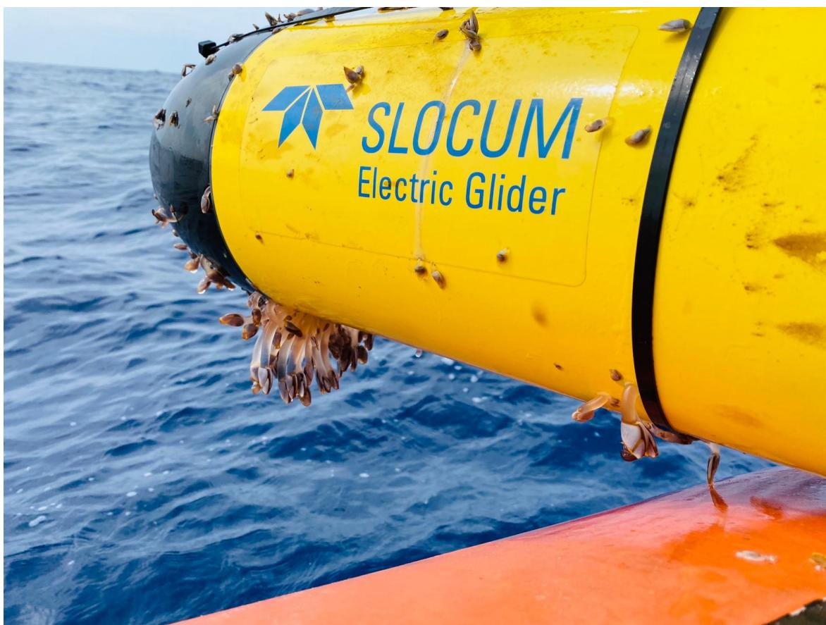
Figure 2.1: Biofouling on recovery
