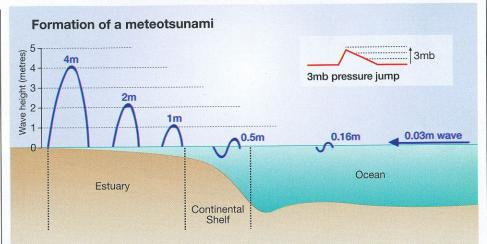
How a meteotsunami forms: a 3mb pressure jump over the ocean causes a 0.03m wave. As it travels, this increases in height by resonance until, finally, at the head of an estuary it can reach up to 5m high
