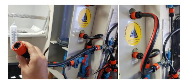
Close tank sink and flush with freshwater until the tank is full. Close "Y" air when filled.
