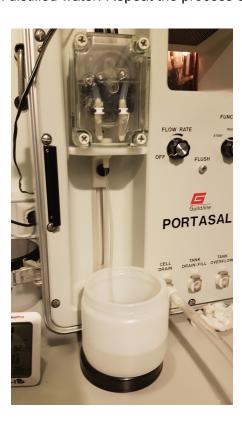
• After the third flush, fill the circuit with distilled water and leave it filled.
