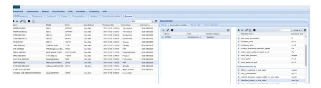
• Set the **associated variables** for each sensor and change the Name according to the NetCDF variable name.
