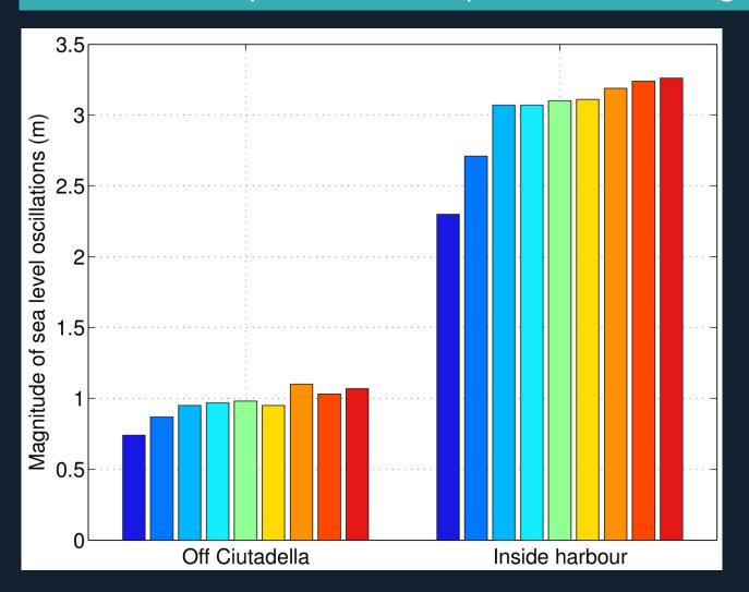
9 WRF simulations using the same setup: rissagues from 2.30m to 3.26m, average 3.00m
