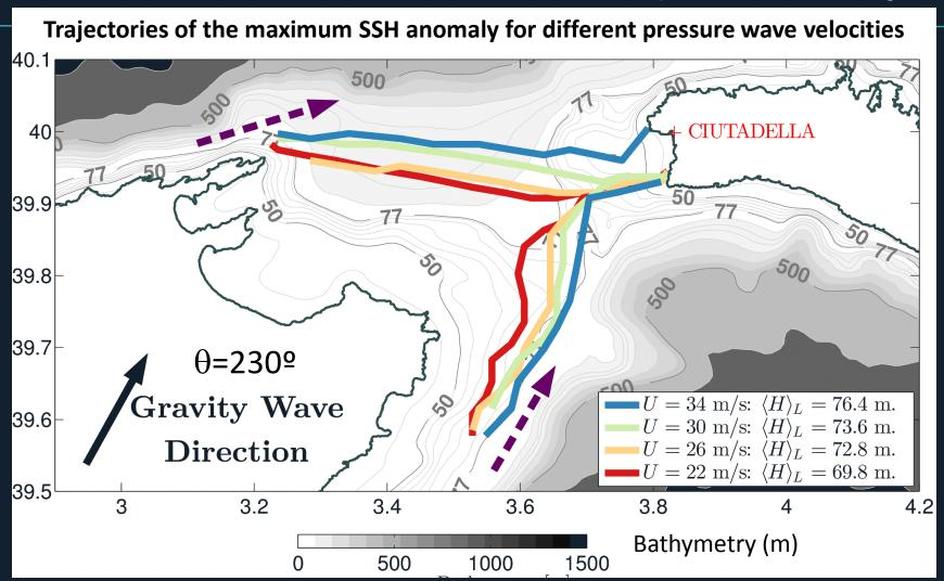
→ Amplification associated with Proudman resonance occurs in deeper water as the atmospheric wave goes faster
