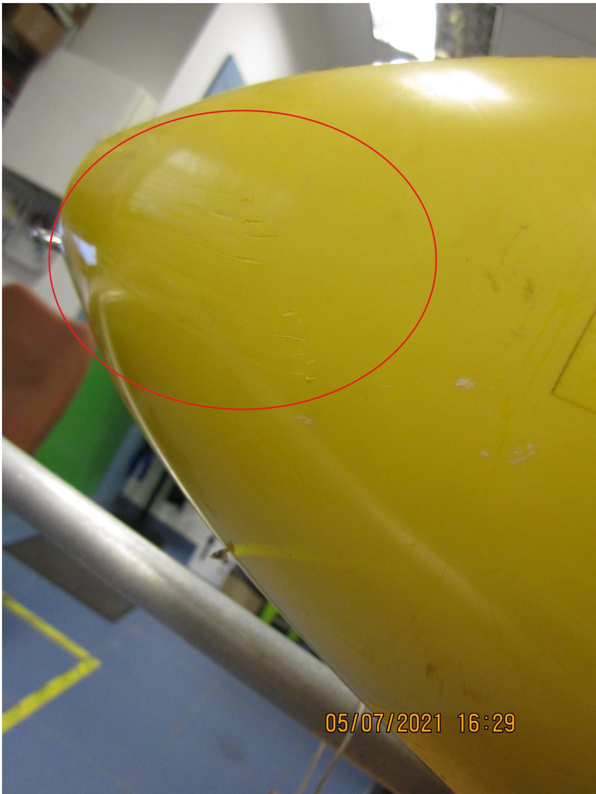
Figure 1.2: Hull Scratches
