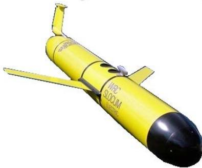
*Figure I.5.1 – Slocum Deep Electric Glider. Manufactured by the Teledyne Webb Research company. Deep models are suited for a maximum depth of 1050 meters while shallow models are limited to 200 meters (although there are version for 30 meters only)*
