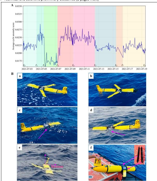
Figure 1. (A) anomaly scores over the test. (B) a: the glider at the beginning of the test, b: the glider before recovery at the end of the test, c: the glider with its left wing removed, d: the glider with its
